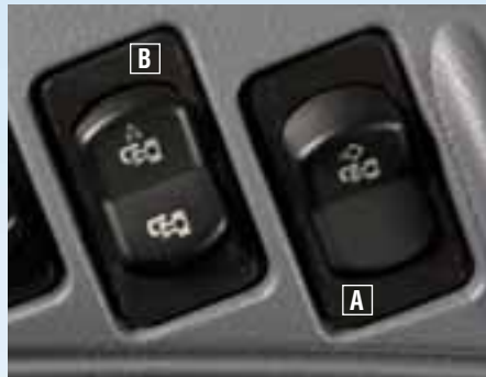
Switches on the right-hand console are used to alert the system that you are ready to record (A) or play back (B) a sequence of actions. Then, press the “step” button to actually activate the recording or play-back. The step button is located on the multi-controller (C) on Elite six-cylinder models, and on the seat-mounted electronic draft control mouse on Elite four-cylinder models.
